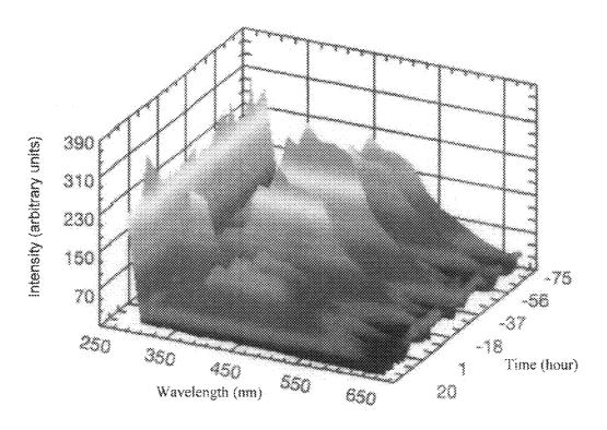
Samples obtained over a five-day research cruise through the Gulf of Mexico. The increased emission due to DOCs near 450 nm was correlated to outflow form river plumes into the Gulf.
