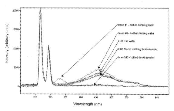
Three brands and tap water are assessed using 266 nm laser excitation. The fluorescence near 450 nm is due to dissolved organic compounds (DOCs) in the water while the small peak near 320 nm is due to leached plastic resins (bisphenol-A).
