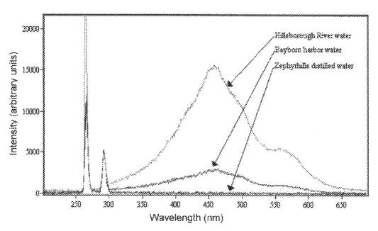
Samples taken from a local river, Tampa Bay and clean distilled water using 266 nm laser excitation. The fluorescence near 450 nm is blue in color and is due to dissolved organic compounds (DOCS) in the water.
