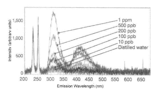
Spectrum shows a dominant peak near 310 nm and a secondary peak near 420 nm form photo-decomposition products.
