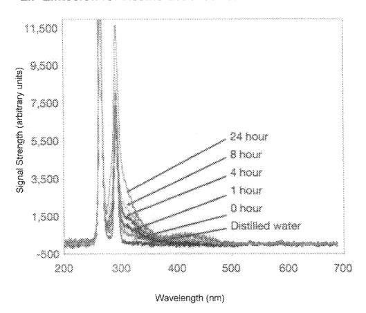
Spectrum of water sample from a plastic food container that was heated for three minutes in a microwave oven.
