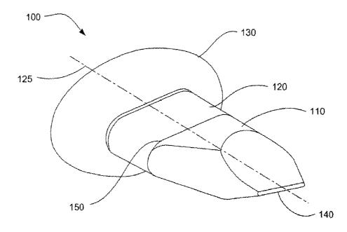
(57) Abstract: Systems and method in accordance with embodiment of the present invention can includes a distractible implant comprising a distracting insert and a body having a first part and a second part adapted to be positioned between adjacent spinous processes of cervical vertebrae. The distracting insert can be inserted into cavities of the body, thereby urging apart the first part and second part, and distracting the adjacent spinous processes.
