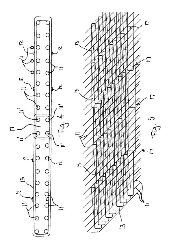
Interlocking Windings without top and bottom carpets Top View
