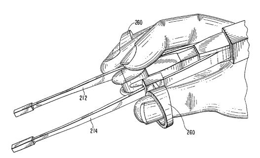
(57) Abstract: A surgical instrument comprises two oppositely-positioned working numbers (212, 214) each having proximal and distal ends and each having a working surface. The instrument also comprises at least one ring member (260) affixed to a least one of the working members to encompass one or more of a user's fingers. In one embodiment at least one working surface has a heating element to cut or seal and cut tissue.
