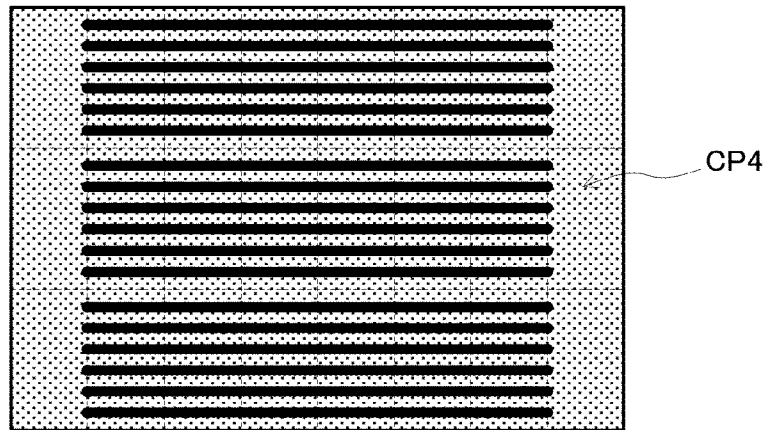
FIG. 11 B PRINT COIL PATTERNS
