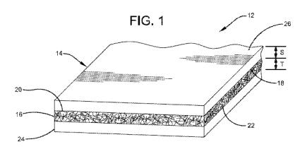
(57) Abstract: A construction composite comprising a construction article having a planar surface and a non-woven layer of pressure-sensitive adhesive disposed on the planar surface.
