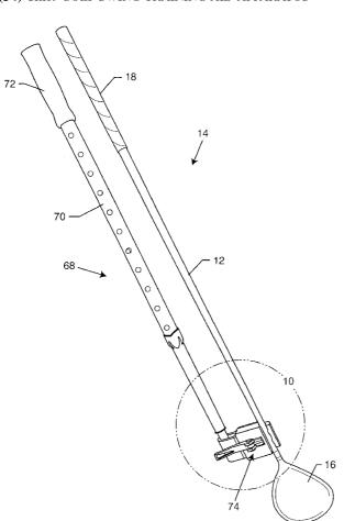
(57) Abstract: A golf swing training apparatus (10) includes an elongated shaft (22) having a clamp (20) attached to an end thereof, which is adapted to be removably attached to the shaft (12) of a golf club (14) so that the training apparatus shaft (22) and the golf club shaft (12) are disposed in spaced apart parallel relation. The training apparatus elongated shaft (2) has first and second shafts slidably disposed for telescopic length adjustment.
