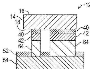
coupled to the intermediate metal layer is reflowed to form an intermetallic layer.
