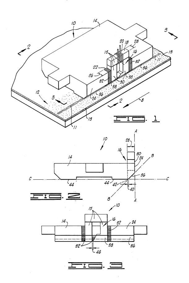
MAGNETIC TRANSDUCER WITH SIDE MOUNTED FERRITE CORE AND METHOD OF MAKING THE SAME
