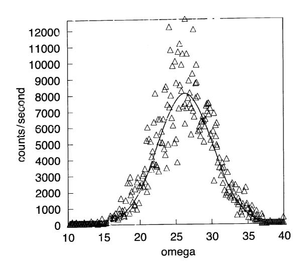
Ni-9at%W-0.03at%Mg alloy Annealing Temperature = 1200°C
