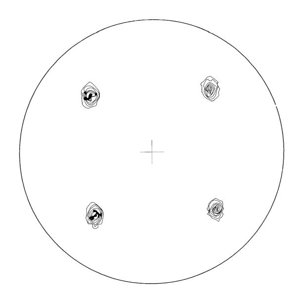
Ni-9at%W alloy Annealing Temperature = 1200°C
