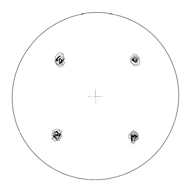
Ni-9at%W alloy Annealing Temperature = 1400°C
