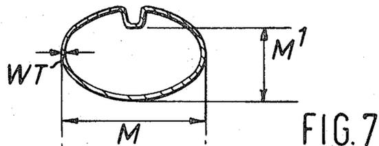
RELATIONSHIP  $A = \frac{M}{WT} = \frac{\text{MAX. EXT. DIA.}}{\text{MAX. WALL THICKNESS}} \geq 26$
