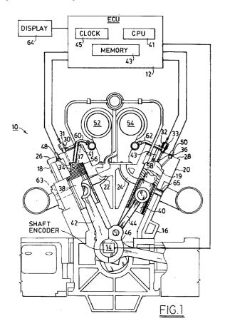
This invention relates to injection timing and power balancing control, e.g. for a two-stroke gaseous fuel engine, and in particular, to controlling the injection timing and output power in each cylinder in response to engine operating conditions and engine type.
