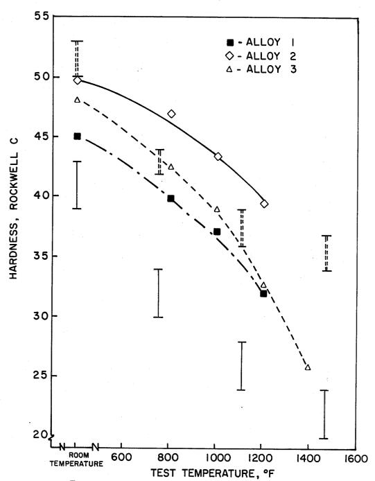
$\underline{I}$  - range for undiluted stellite 6 weld deposits (ref. 1)
