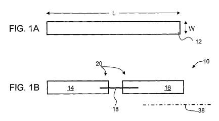
(57) Abstract: A rectifying antenna device is disclosed. The device comprises a pair of electrode structures (14,16), and at least one nanostructure diode (12) contacting at least a first electrode structure of the pair and being at least in proximity to a second electrode structure of the pair. At least one electrode structure of the pair receives AC radiation, and the nanostructure diode (s) (18) at least partially rectifies a current generated by the AC radiation.
