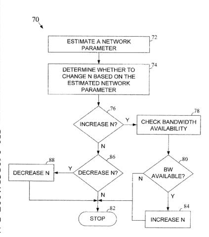
(57) Abstract: A multicarrier communication device can vary the number of subcarriers being used to carry on multicarrier communication within a network, based on a predetermined criterion (e.g., traffic load, etc.).
