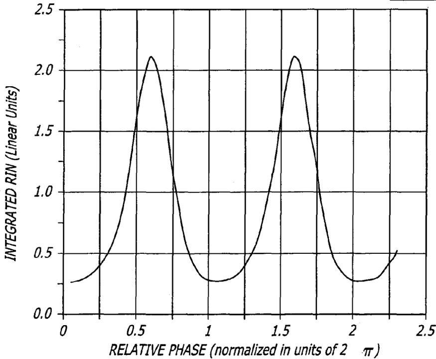
— Integrated RIN over selected bandwidth (for an External Cavity Length used during our Reduction to Practice)
