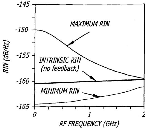
— Intrinsic RIN of Diode Laser (no external feedback applied)
