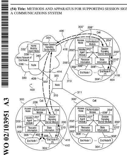
(57) Abstract: A mobile network (Fig. 4) which uses SIP, Mobile IP and RSVP:
