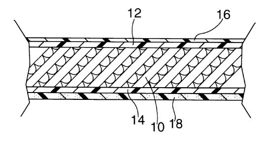
The invention relates to a release liner with a flat base substrate coated on both sides with thermoplastic polyolefin
