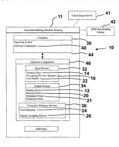
(57) Abstract: An automated banking machine system and method includes ATMs (11) which accept checks (26) and dispense cash (24) to users. The ATMs are operated to acquire image and magnetic data from deposited checks to determine the genuineness of checks and the authority of a user to receive cash for such checks. Cash may be dispensed to the user from the ATM in exchange for the deposited check The ATMs dispense cash to communications with a transaction host.
