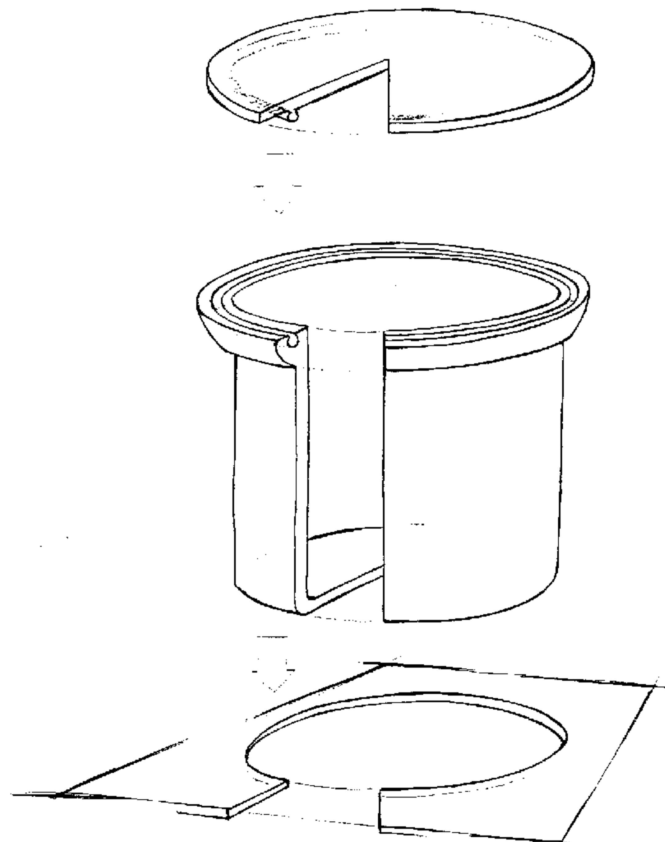
(57) The invention relates to a device for molecular and macromolecular crystallization. More particularly, the device comprises a well and a transparent cap for growing diffraction-quality protein crystals by conventional vapor diffusion techniques. The present device is particularly advantageous in that it allows the pre-filling of the well with a solution for transport and handling.
