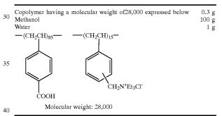
A photosensitive liquid 1 described below was prepared. The resultant substrate was coated with the photosensitive liquid 1 so that a coating amount thereof was 1.3 g/m<sup>2</sup>, thereby obtaining a planographic printing plate 1. Photosensitive Liquid 1
