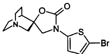
**25** *(R)-3'-(Thiophen-2-yl)spiro[1-azabicyclo[2.2.2]octan-3,5'-oxazolidin]-2'-one* (425 mg, 1.61 mmol) and *N*-bromosuccinimide (287 mg, 1.61 mmol) were stirred in DMF (7 mL) at 80 °C for 3 h. The mixture was allowed to cool to room temperature, and was then diluted with chloroform, washed with aqueous potassium carbonate, then with brine, then
