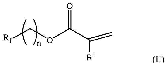
15      wherein  $\text{R}_f$  is  $\text{C}_2$  to  $\text{C}_{10}$  fluoroalkyl, optionally interrupted by one or more  $-\text{O}-$ ,  $-\text{CH}_2-$ ,  $-\text{CFH}-$ , or combinations thereof,  $n$  is an integer from 1 to 10, and  $\text{R}^1$  is  $\text{H}$  or  $\text{CH}_3$ . Examples of  $\text{R}_f$  include, but not limited to,
