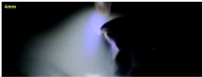
Mov. 3.5 Arc bypass phenomenon (Slow motion)
