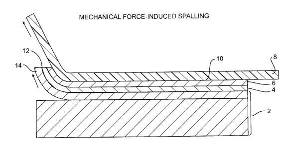
PARENT SUBSTRATE (Si, Ge, GaAs, SiC) (SINGLE OR POLY CRYSTAL)(ANY ORIENTATION)
