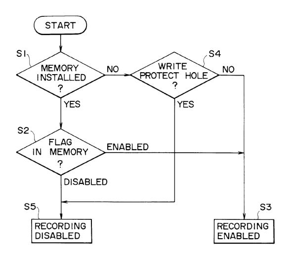
RECORDING / REPRODUCING APPARATUS COMPATIBLE WITH MEMORY-BASED RECORDING MEDIUM CASSETTE
