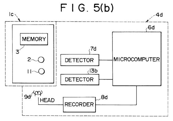
RECORDING / REPRODUCING APPARATUS INCOMPATIBLE WITH MEMORY-BASED RECORDING MEDIUM CASSETTE
