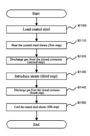
internal pressure through variable control of the amount of steam flowing into said closed container (10) and/or the amount of steam flowing out of said closed container (10), and in said closed container (10) that can maintain said predefined pressure, said Zn—Al—Mg alloy coated steel sheets (1) have contact with the steam introduced into said closed container (10).
