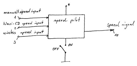
(57) Abstract: The adaptive speed control system comprisis a speed pilot by which the speed of an automobile can be automatically hold at a first speed value. Said speed pilot is connected to an information system in which maximum speed limit information is stored. A control system is provided for changing the first speed value into a second speed value corresponding to the maximum speed limit information.
