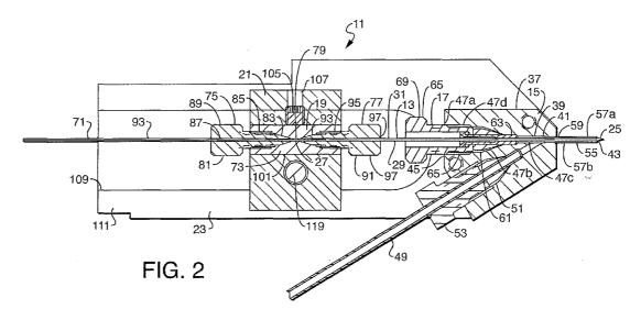
(57) Abstract: Embodiments of the present invention facilitate servicing or changing a discharge tube or modifying the position of a discharge tube with respect to a orifice of a detector and/or a nebulizing gas conduit. The apparatus features a discharge tube housing that slidably receives a discharge tube. A union coupling the discharge tube to a source of fluid is slidably mounted to a mounting assembly holding the tube housing.
