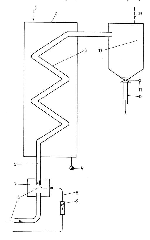
heat exchanger for example. It is accordingly very easy to clean, and there are no dead spaces in the exchanger for the mass to remain in too long.
