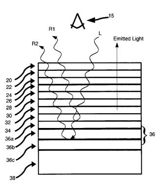
(57) Abstract: An contrast enhanced OLED device is provided that has a layer of lithium fluoride or lithium oxide deposited within the stack of the device. The lithium fluoride or lithium oxide is deposited in addition to, or in conjunction with, one or more contrast enhancement layers that are also within the stack of the device.
