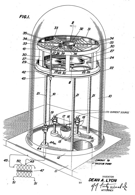
METHOD FOR COATING OPTICAL ELEMENTS
