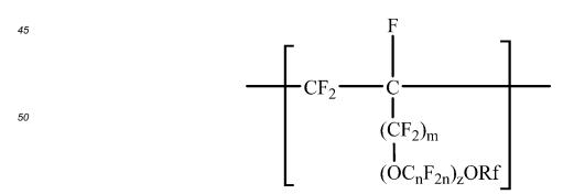
are present in the copolymer according to the present disclosure in a combined amount from 0.02 mole percent to 2 mole percent, based on the total amount of the copolymer. In some embodiments, the copolymerized units represented by these formulas are present in the copolymer in a combined amount up to 1.5 mole percent or up to 1.0 mole percent.
