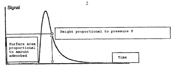
[0011] FIG. 1. Principle of determining a point of the adsorption isotherm at relative vapor pressures p/p0 in the range of 0.01 < p/p < 0.3.
