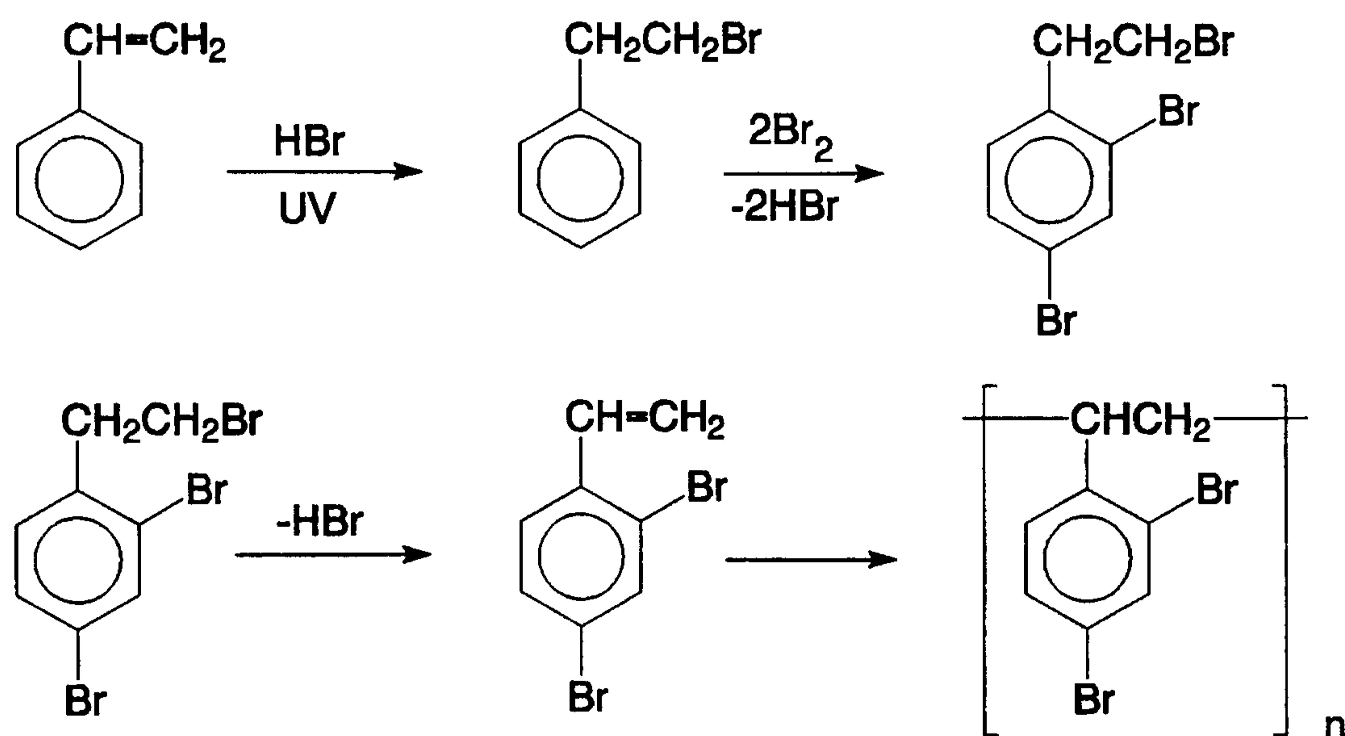
20        This process has one significant advantage. It produces a brominated polystyrene which is essentially free of backbone halogen. This results in a product with very good thermal stability, good color, and good color stability.
