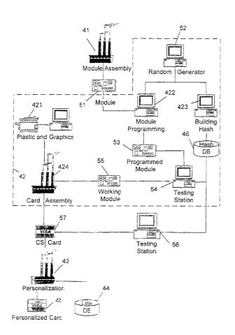
(57) Abstract: A method of manufacturing an identification card (10). The method includes providing a substrate (17) carrying a circuit including at least one electronic element (12) and laminating the substrate to at least one isolating layer (25), using an at least partially hot lamination process, so as to form a card (10).
