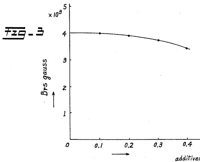
Fig. 2 polyvinyl chloride-acetate copolymer-polyurethane resin + additives.
