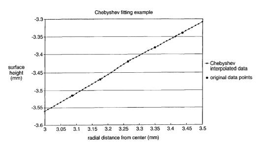
(57) Abstract: The invention provides a method for designing lenses and lenses produced thereby in which method locally fitted Chebyshev polynomials are used to design one or more of the lens' surfaces.
