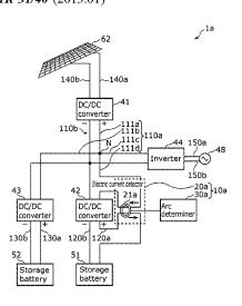
currents detected by the electric current detector, whether an electric arc has occurred.
