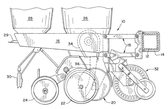
(57) Abstract: A seed tube (36) for an agricultural seeding machine (10) includes a side wall (42) having at least a portion thereof (52) formed from a transparent material. A sensor (54, 56) includes a transmitter (54) which is positioned adjacent an outside of the side wall (42), and operates through the transparent material (52).
