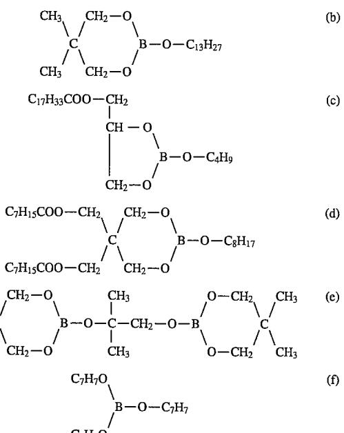
The borate ester compound used in these examples were prepared by reacting the following alcohols with one mole of boric acid for condensation:
