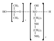
in which x and y are integers which depend on the molecular weight, the average molecular weight being approximately between 5,000 and 10,000. This polymer is also known as "amodimethicone".
