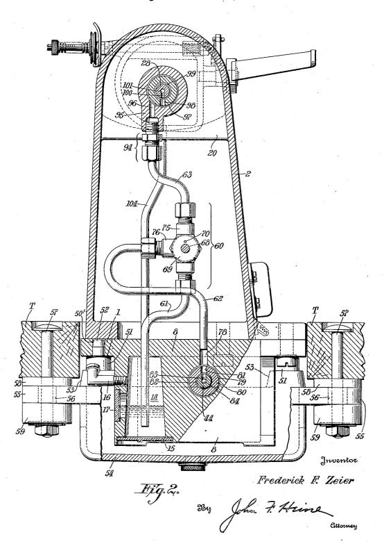
LUBRICATING SYSTEM FOR SEWING MACHINES
