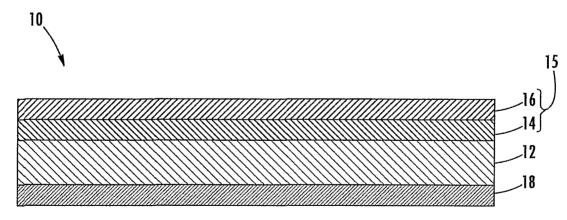
(57) Abstract: An ink-jet printable medium (10) includes a substrate (12) having an imaging surface with a supporting intermediate coating (14) overlying the imaging surface and a microporous ink-receptive coating (16) overlying the supporting intermediate coating (14).
