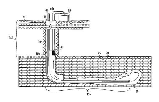
(57) Abstract: A method an apparatus for solution mining using a single well. Fluid (55) is injected by conduit (45). Solution is produced through casing (60b) external to the conduit (45). Fluid may be heated, and may be caustic.
