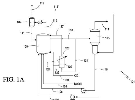
(57) Abstract: The present invention relates to improved processes for the manufacture of acetic acid. A pump around reactor is used to produce additional heat for the production of steam. The pump around reactor receives a portion of the reaction solution produced by the carbonylation reactor and further reacts that portion with additional carbon monoxide and/or reactants.
