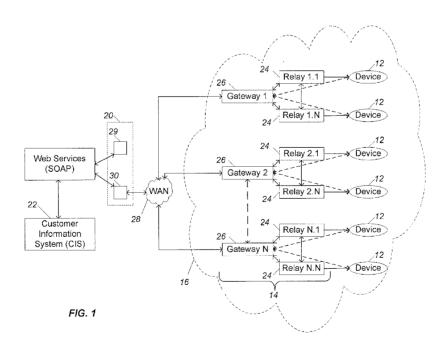
(57) Abstract: A system associated with a utility network having product distribution pathways, including a device management module for automatically provisioning at least a subset of a plurality of electronic utility devices associated with the pathways based on configuration state information received from the subset of the plurality of electronic utility devices and a comparison of the received configuration state information and predefined configuration state information.
