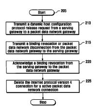
PDN type associated with the PDN connection is an IPv4/v6, which indicates that the UE is allocated both the IPv4 address and the IPv6 address; the PGW transmits, to a Serving GateWay (SGW), a Binding Revocation message including information indicating release of the IPv4 address with the PDN connection remaining if the PDN type is the IPv4/v6; and the PGW receives, from the SGW, a Binding Revocation acknowledge message to acknowledge release of the IPv4 address.
