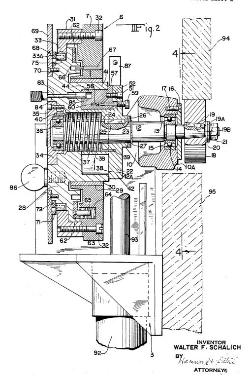
STRETCH GAUGE MEASURING AND STRETCH STROKE LIMITING DEVICE
