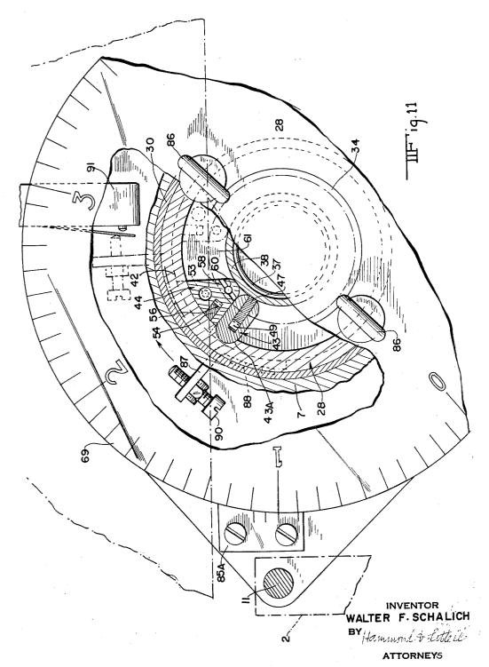
STRETCH GAUGE MEASURING AND STRETCH STROKE LIMITING DEVICE
