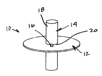
(57) Abstract: An information media holder assembly (10) includes an information media storage element (12) supported on an information media storage element support (14). The information media storage element support (14) has a storage element retention mechanism (16) adapted to receive and retain the information media storage element (12) and a novelty mechanism (18) unrelated to information media storage element retention.
